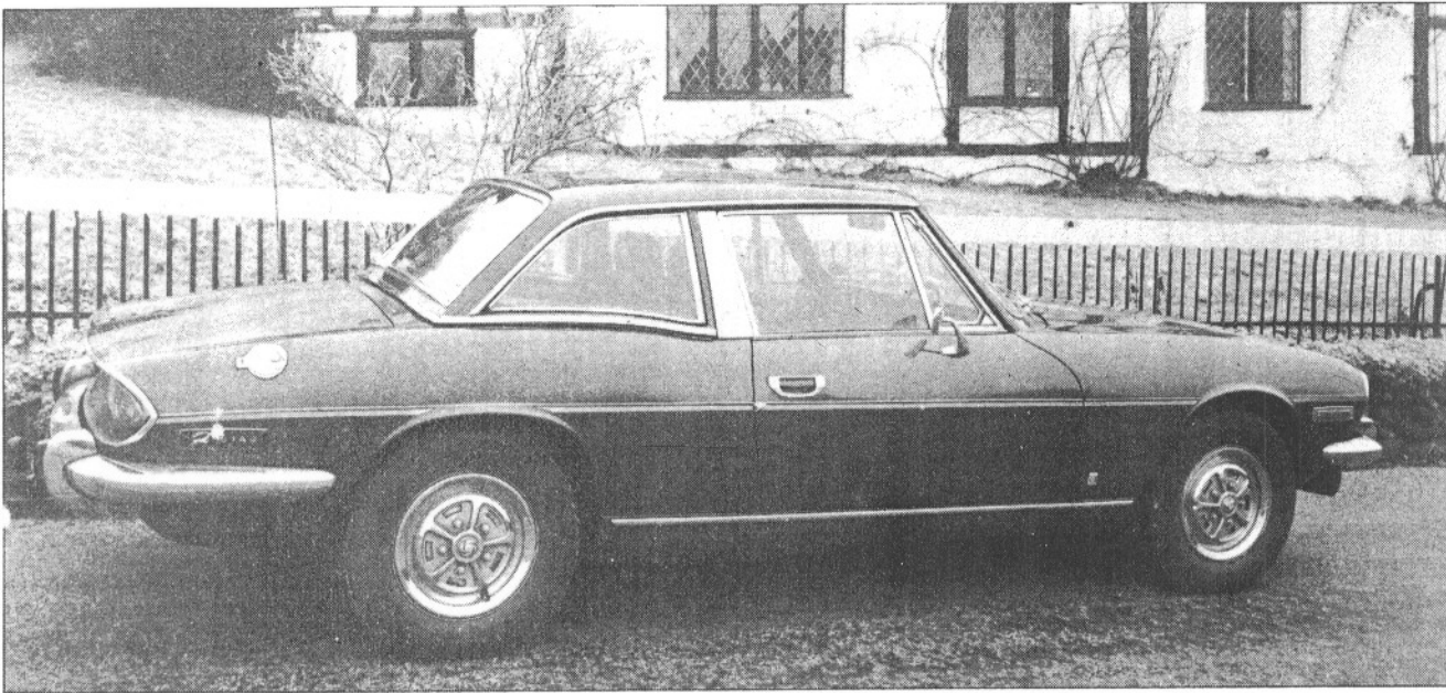
Left. The hard top gives closed car comfort but there is some extra wind noise from the screen top joint. Below. Four-way adjustment of the steering column, in-out and up-down
