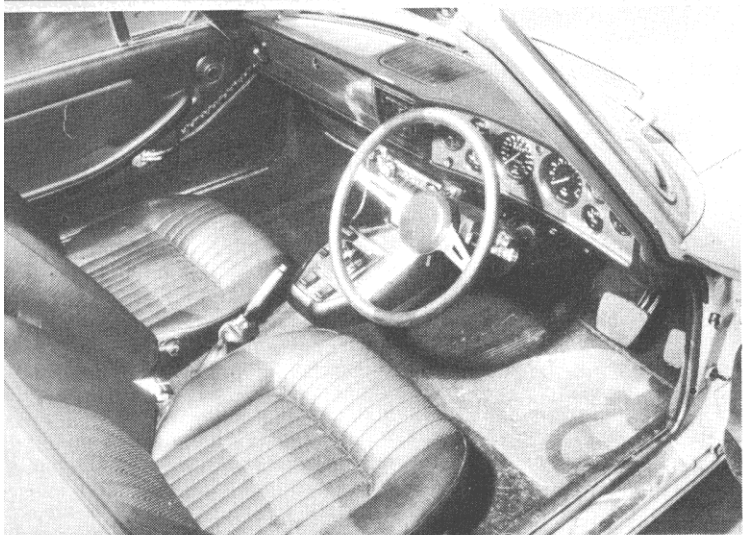
Above: the sumptuous seats lack thigh support despite the facility of a built-in cushion tilt. Top right: a smaller diameter wheel and less assistance give more feel to the steering. Below left: the built-in roll cage not only offers protection but stiffens the framework as well. Below right: entry to the rear is awkward and headroom limited. The seat, however, is comfortable
