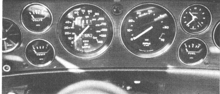
The comprehensive instrumentation is easy to read and well-sited. We query the fitting of a battery condition meter in preference to an oil pressure gauge
