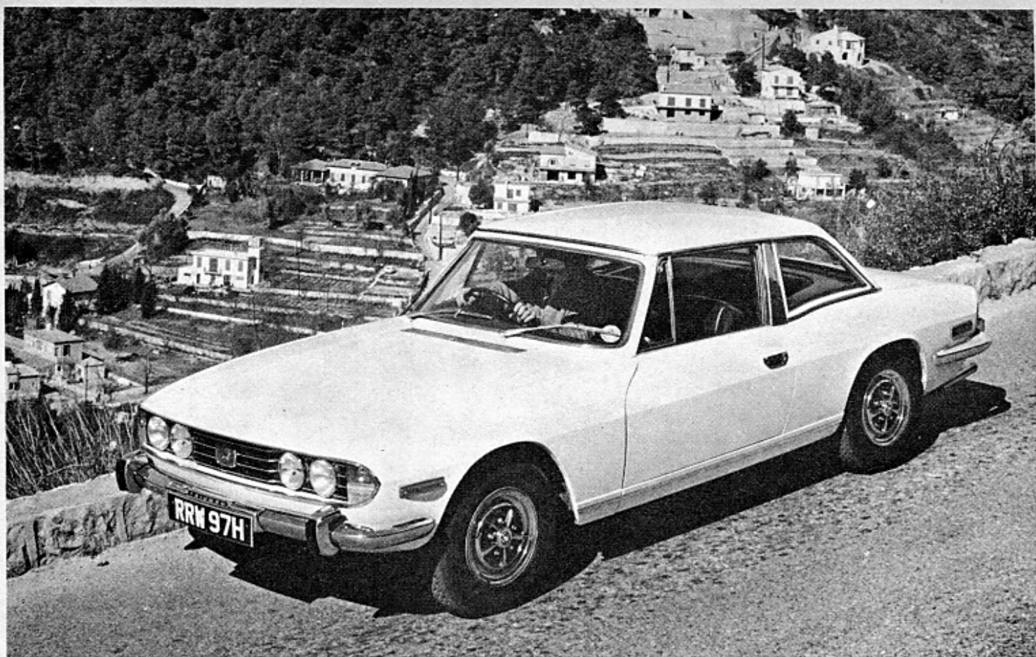
The new Triumph Stag's 2 plus 2 body is available either as a soft top or with a detachable hard top.
