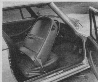
Below: The front seats are released by a catch high up on the door side, tipping slightly sideways as well as forwards to permit access to the back seat
