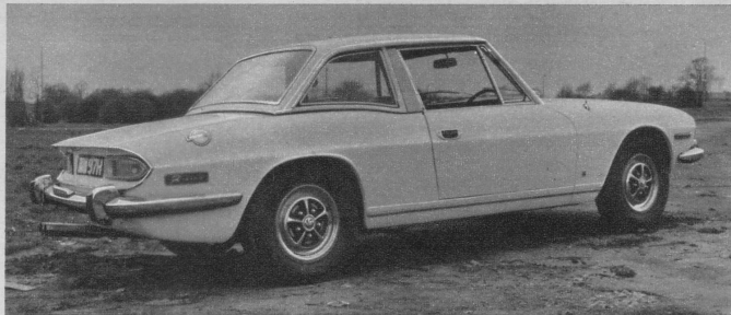
Above: The three-quarter rear view, with the hardtop in position, again betrays a relationship with the saloons. The hardtop is well endowed with window area; the rear quarter windows hinge open at their leading edges, and the rear screen is electrically heated
