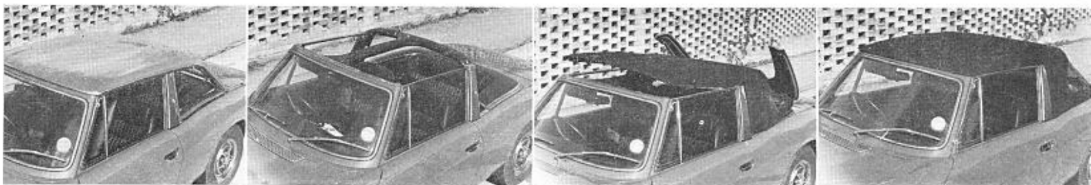
Hard-top to soft-top in 1 min. 36 sec. L. to r.: hard-top fitted; top off, hood down showing roll-over structure (42 sec.); erecting the previously hidden hood (54 sec.); soft-top erect.
